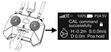
*Step 2*: When the screen shows "Horizontal calibration", hold the drone horizontally with its nose outwards and start rotating. The RC will emit a long beep indicating the horizontal calibration has succeeded.
