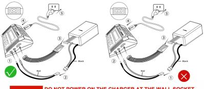
WARNING DO NOT POWER ON THE CHARGER AT THE WALL SOCKET UNTIL THE CABLES ARE ALL CONNECTED PROPERLY
