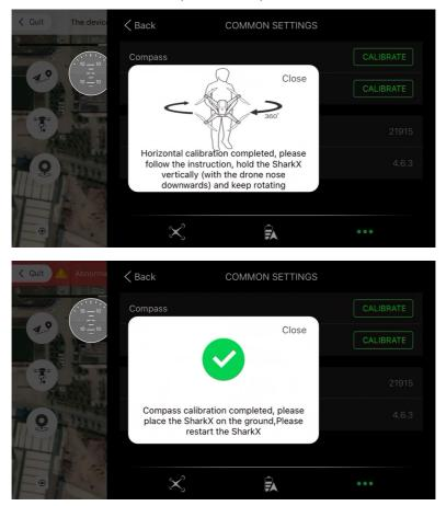
Notice calibrate the compass when there are no less than 15 satellites
