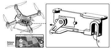
0. Press the 'Release Switch' button on the remote control to open the hook release mechanism.
