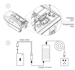
Direct charging: 5.5/2.5 DC charging port (*please refer to Picture1*). Please note that both batteries must be inside the boat together when direct charging. It takes 4-6 hours to be fully charged; or
