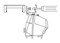
Step 2 Install the antenna
