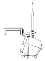
Step 3 Attach your mobile device to the mobile device holder clamp
